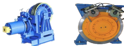
Asynchronous motor Synchronous motor
